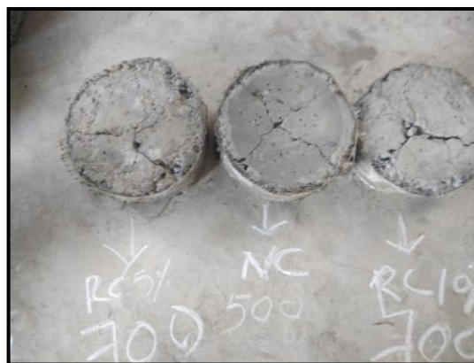
Figure 26: specimens with GFRP sheets after impact test
