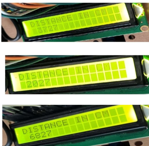
Fig 5: LCD display showing the distance of the obstacle measured by the robot
